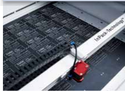
The InPack Technology™ protects the axis against dust and dirt
